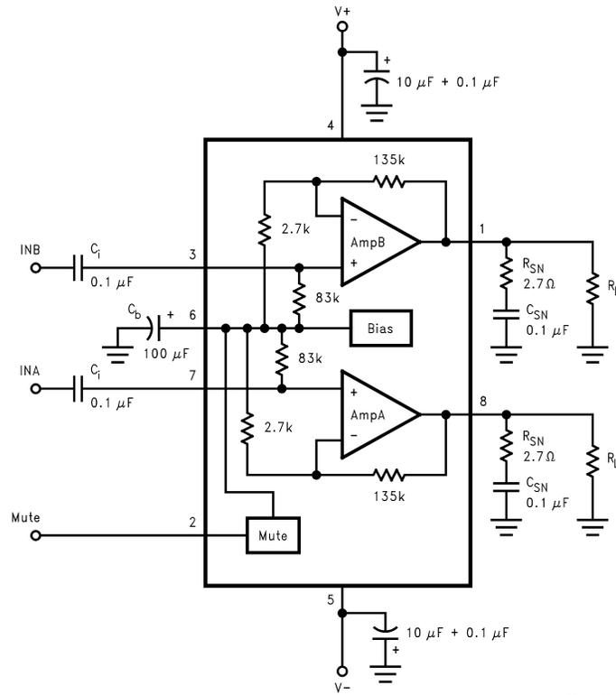
FIGURE 2. Test Circuit
