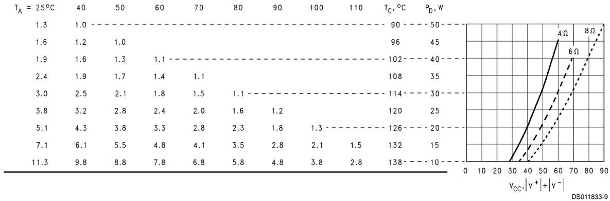
**Note:** The maximum heat sink thermal resistance values,  $\theta_{SA}$ , in the table above were calculated using a  $\theta_{CS} = 0.2^\circ\text{C/W}$  due to thermal compound.
