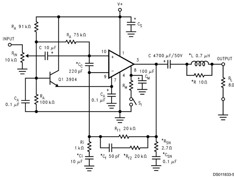
\*Optional components dependent upon specific design requirements. Refer to the External Components Description section for a component functional description.
